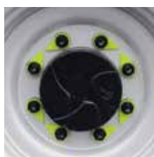
Indicators for loose nuts
