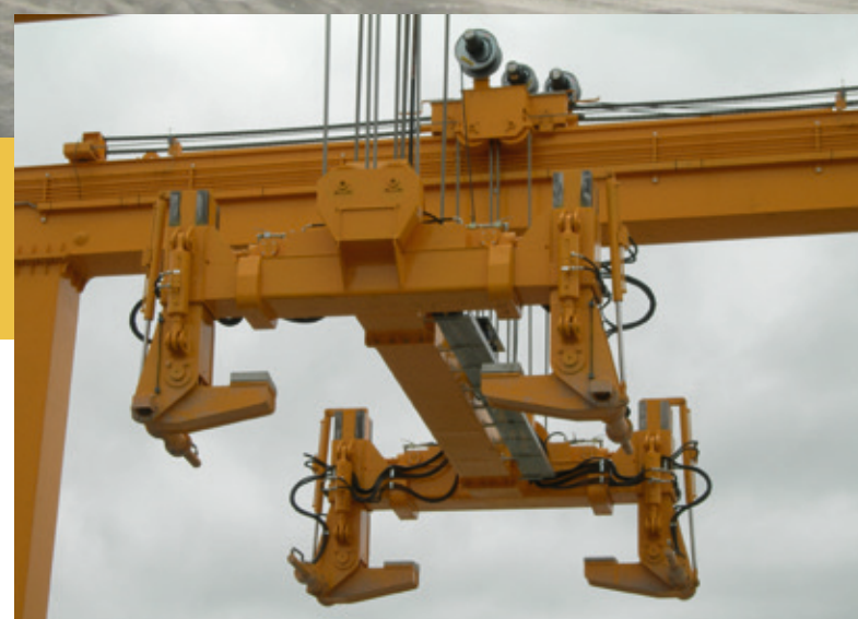
Special hydraulic clamps for concrete segments
