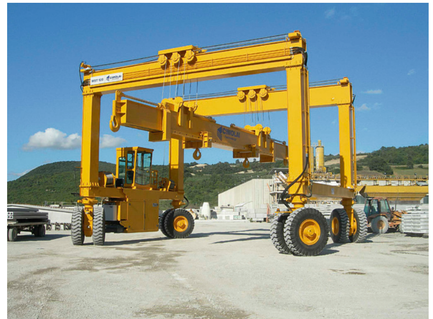
Capacity: 120 t ITALY Hydraulic telescopic spreader
