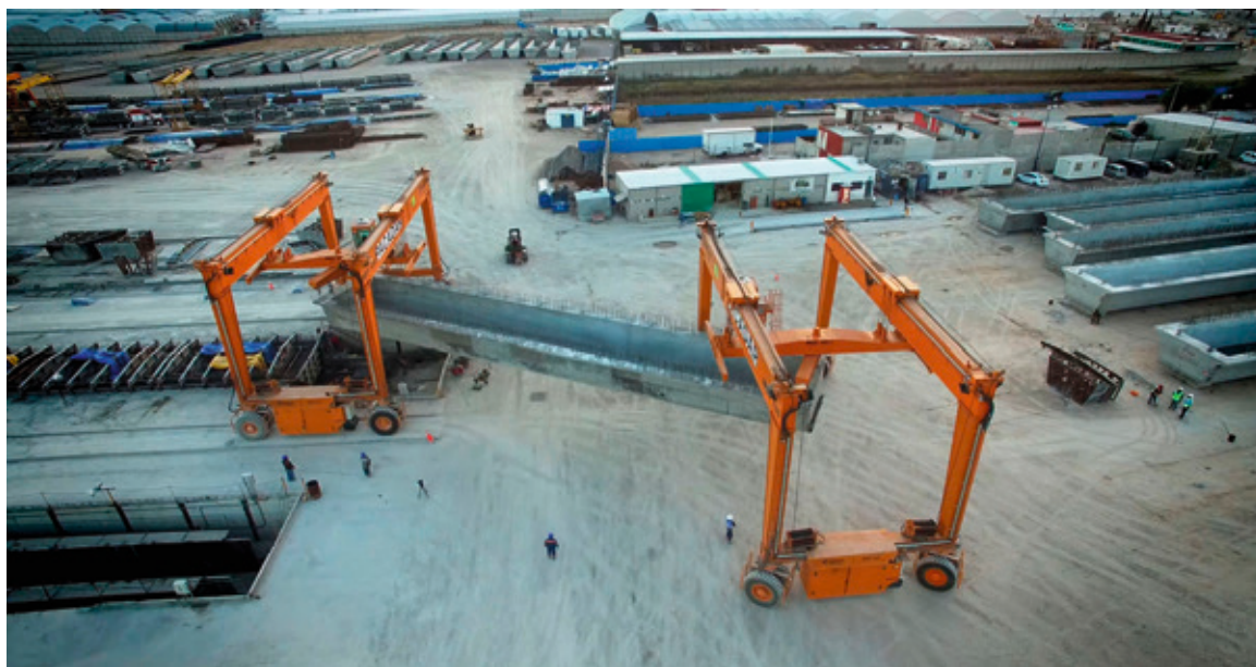
Capacity: 135 t/each MEXICO N.2 units also suitable to be used in tandem
