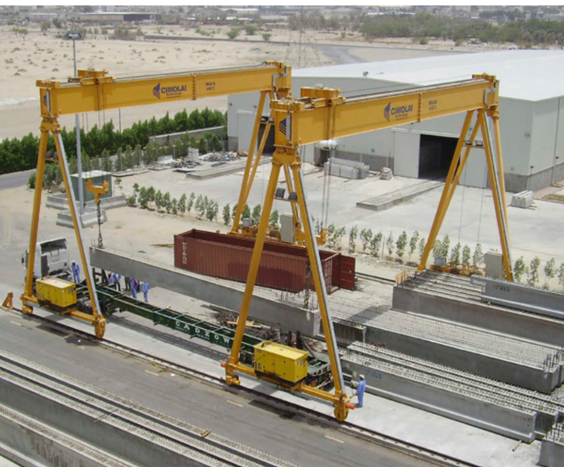
Capacity: 40 t/each - SAUDI ARABIA Single girder version with generating set
