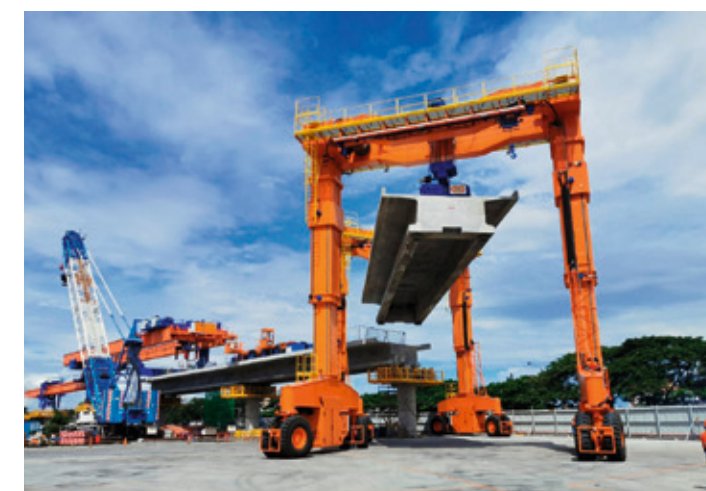
N.2 units single girder version suitable to be used in tandem
