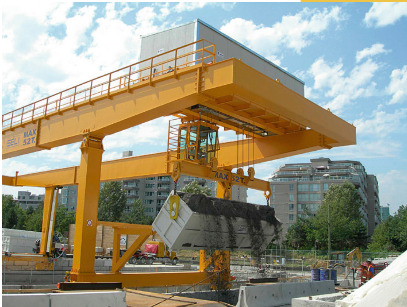
Capacity: 52 t - CANADA Special system to unload digged material
