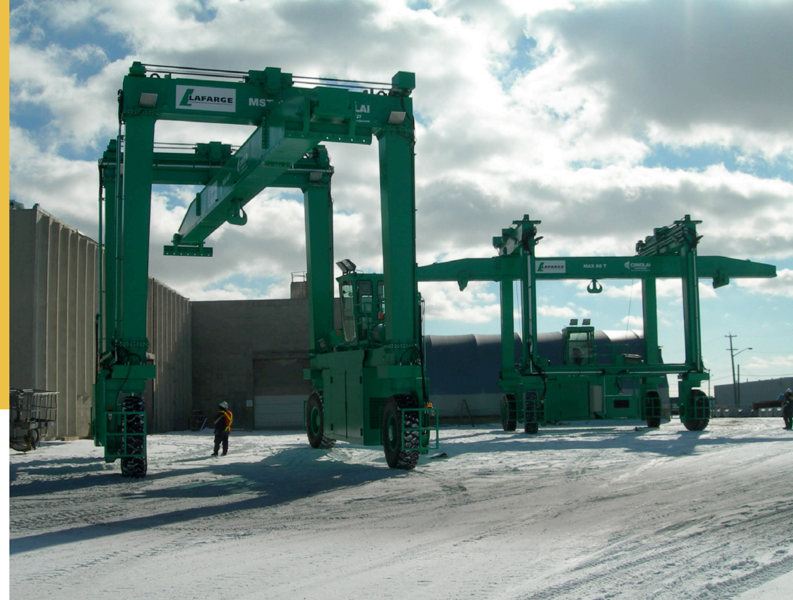
Capacity: 100 t /each - CANADA - N.2 units suitable to work at -40°C
