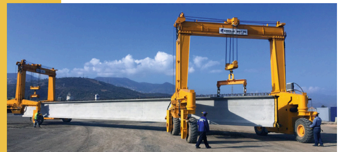
Capacity: 30 t/each ALGERIA N.2 units single girder version suitable to be used in tandem
