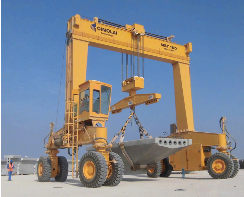
Capacity: 160 t - QATAR - Single girder version
