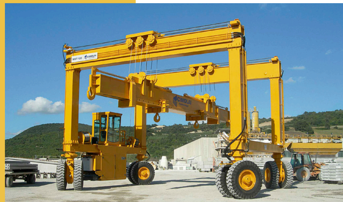
Capacity: 120 t ITALY - Hydraulic telescopic spreader
