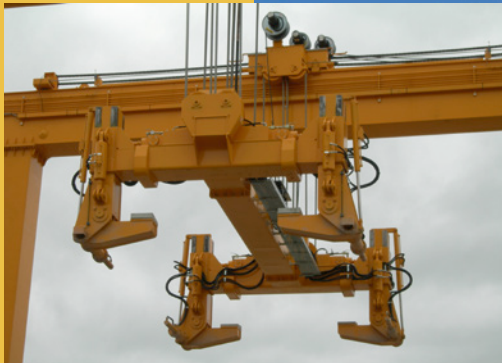
Special hydraulic clamps for concrete segments
