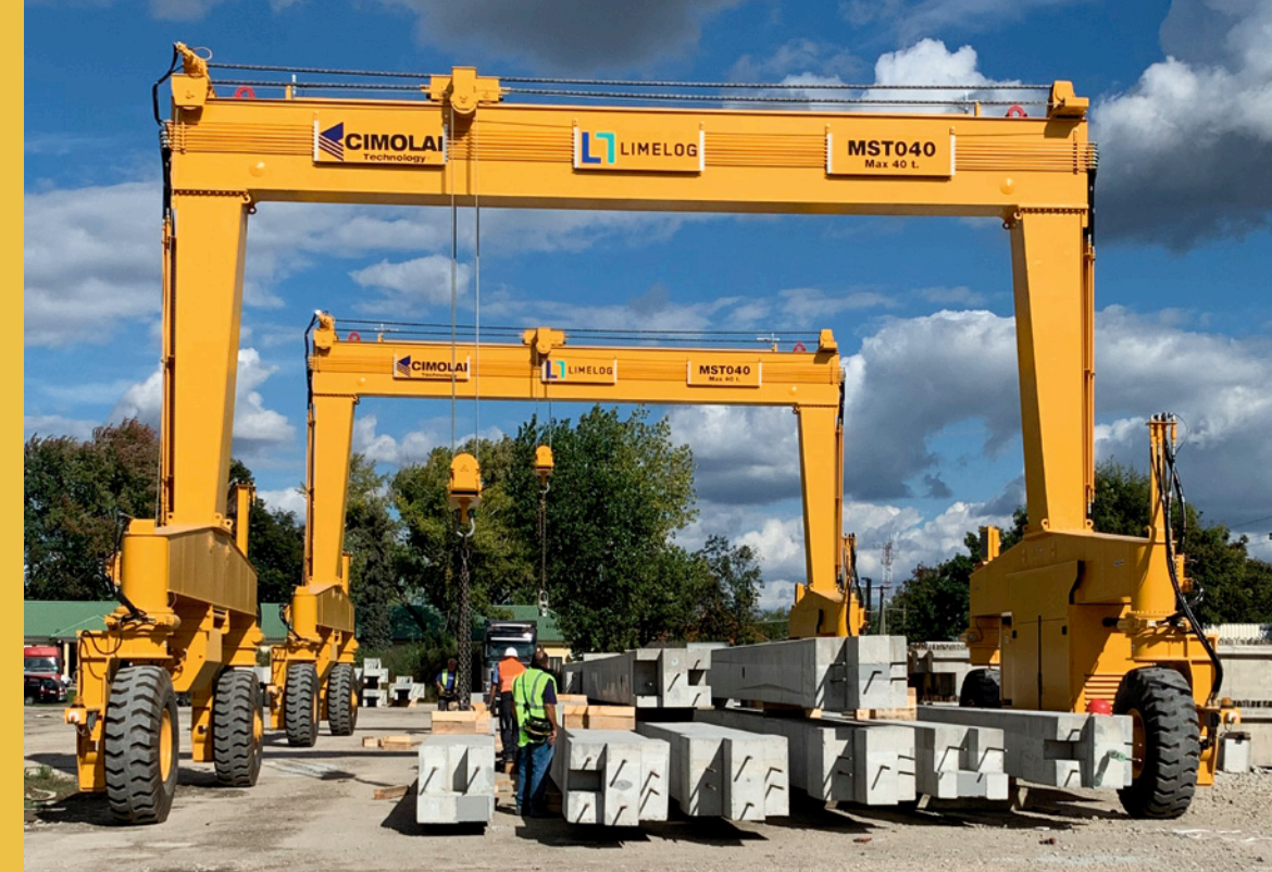
Capacity: 40 t/each HUNGARY N.2 units single girder version suitable to be used in tandem
