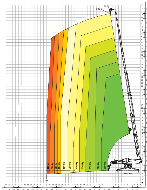
Load chart with Winch 8,000 kg
